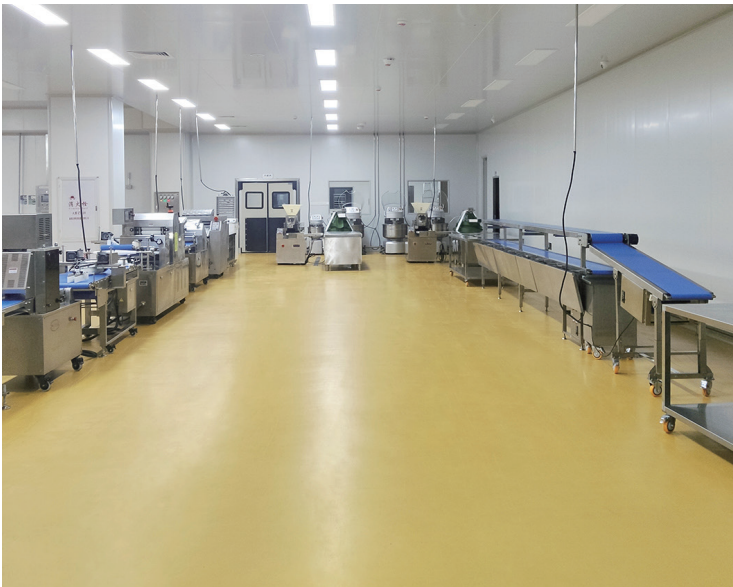
Waterborne Polyurethane Mortar Self-Leveling System 4-6mm
