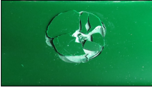
Epoxy: cracks after 3 drops from 1 m
