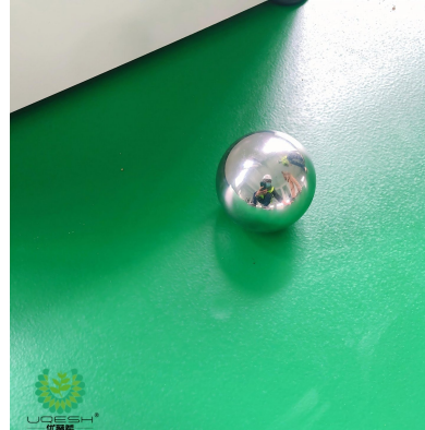
UQESH: 70 drops from 1 m / 10 drops from 2 m, no damage
